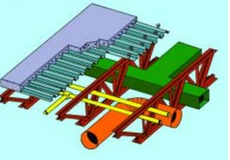
the 26-story 312 EIm Street building in Cincinnati. The lower 10 stories, covering 410,000 sq. ft, used cast-in-place concrete for the parking garage. Composite joists spanning 48.5' supported the upper 16 steel-framed office floors, which covered 326,000 sq. ft. The project had a 16-month construction schedule and \$60-million budget.
